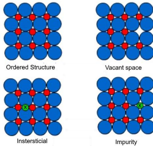
**Figure 1. The trace elements are found inserted into the crystalline networks of the mineral species which make up the rocks of a mined deposit.**
